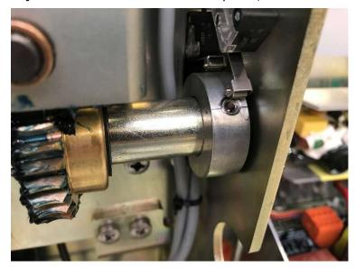
Adjust the cam on the barrier arm on the hill side as shown on the photo.
