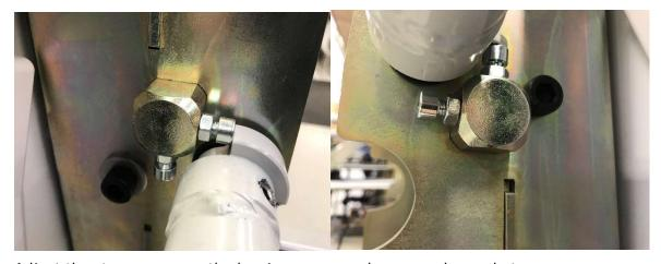
Adjust the stop screws on the barrier arms, as shown on above photos.
